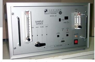
gas can be as high as 5 to 10 ppm. Other contaminants include water vapor and Carbon. These Oxygen Monitors and Inert Gas Purifiers help overcome these issues and are designed for both laboratory size and full production use.
