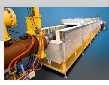
custom-designed furnaces available today. The single or double-ended varieties of this furnace offer semi-continuous operation in a high-vacuum environment, with loads up to 1000kgs in size, and offers faster turnaround time and throughput.
